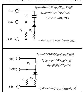
Figure 5 - Guard Time Adjustment
