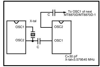
Figure 7 - Oscillator Connection
