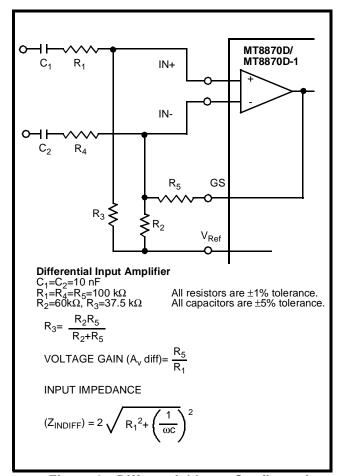
Figure 6 - Differential Input Configuration
