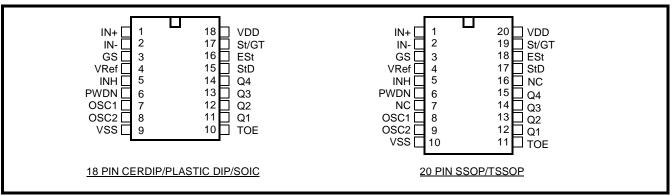
Figure 2 - Pin Connections
