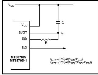
Figure 4 - Basic Steering Circuit
