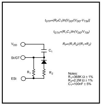
Figure 8 - Non-Symmetric Guard Time Circuit
